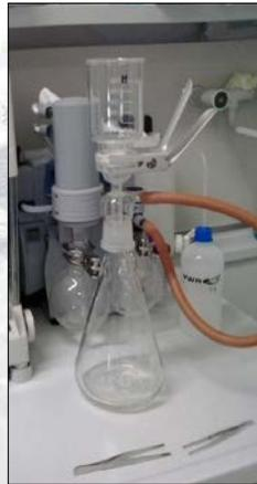
**Filtration** by Whatman filter No. 1 through a vacuum filtration system
