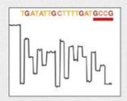
The adapter molecule keeps bases in place long enough for them to be identified electronically.
